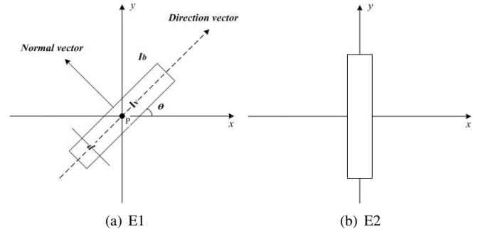
Fig. 1. Vessel modeling: (a) initial coordinate system (E1); (b) coordinate system after alignment on the y axis (E2)
