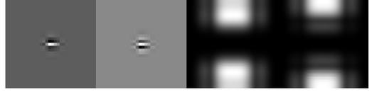
Fig. 5. The first two images show two kernels extracted from the operator  $(\mathbf{W}_1^1)'(\mathbf{W}_1^1)$  where  $\mathbf{W}_1^1$  computed by the standard DWT with db4 wavelet filters. For good visualization, only center part of images ( $32 \times 32$ ) is given. The last two images are the corresponding frequency magnitude responses. Note that the DC component of Fourier transform is located at the center of each image.
