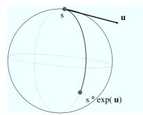
Figure 4: Schematic view of the intrinsic update step used in Newton methods for Lie groups. An unconstrained update u is computed on the Lie Algebra and is projected back onto the Lie group through the exponential map.
