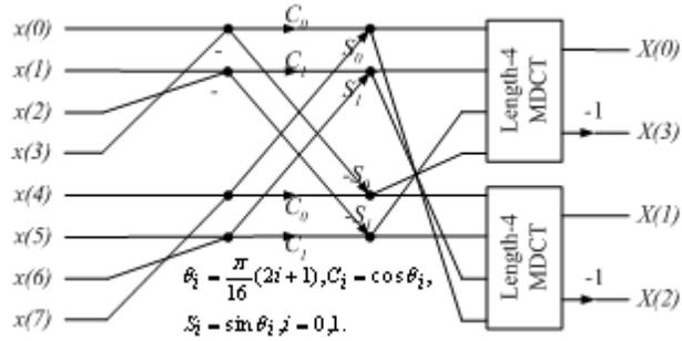
Fig.1. Flowgraph of a length-8 MDCT (*radix-2 DIF*)
