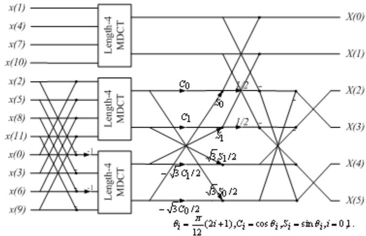
Fig.2. Flowgraph of a length-12 MDCT (*radix-3 DIT*)
