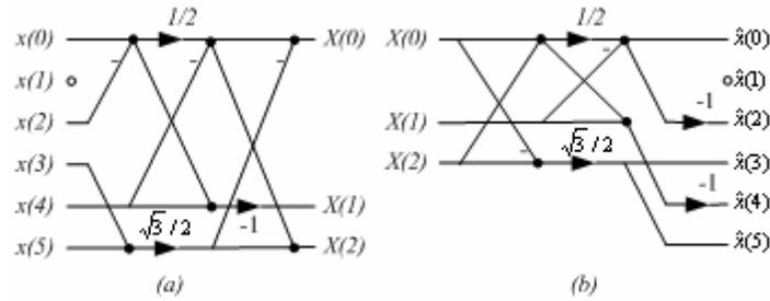
Fig.5. Flowgraph of a length-6 MDCT (a) and a length-6 IMDCT (b).
