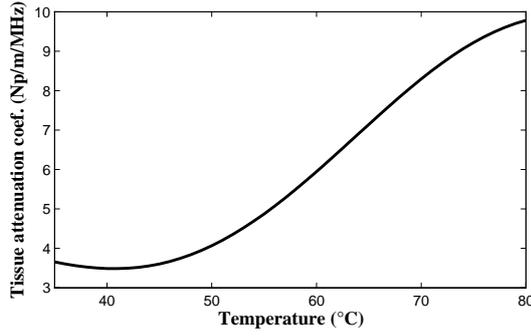
**Fig. 2.** Linearized tissue attenuation coefficient vs. temperature.
