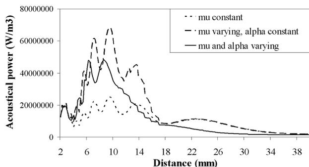
**Fig. 4.** Acoustical power along the axial direction.
