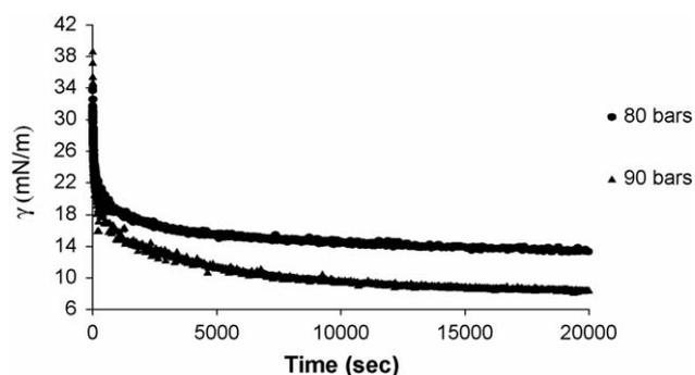
Fig. 8. Kinetics of HSA adsorption at water–CO<sub>2</sub> interface.
