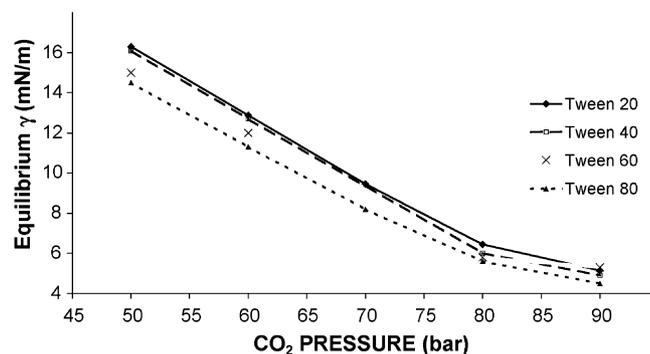
Fig. 5. Equilibrium  $\gamma$  vs. CO<sub>2</sub> pressure for the four types of Tween<sup>®</sup>.
