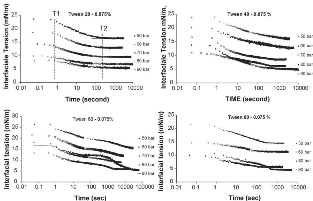
Fig. 4. Kinetics of  $\gamma$  decrease in presence of Tween<sup>®</sup> 20, 40, 60, and 80 at a bulk water concentration of 0.075%. The measurements were performed at pressures ranged from 50 to 90 bar and at a temperature of 40 °C.
