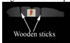
Fig. 1. MR axial image of pig liver. Used as spatial references for axial images, two wooden sticks are clearly identifiable as hypointense. Temperatures were calculated relative to a reference scan before treatment. Thermal maps (colors) were superimposed over the baseline morphological image (grey scale). This is representing temperature increase compared with those at the start of experiment.
