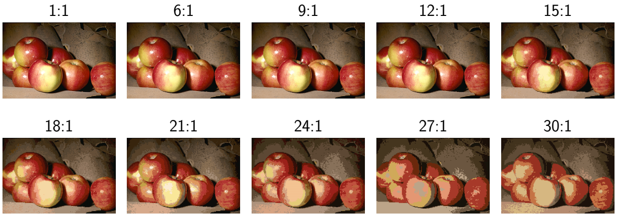
Fig. 1. ((Color online) The effects of VQ compression. The original image (0% compression) is shown after VQ compression using a codebook based on the LBG algorithm applied to the image encoded in the color space L^*a^*b^* (see text). Larger compressions lead to evident decreases in image quality.
