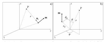
Fig. 4. Coordinate systems. (a) Coordinate system for a dipole in the infinite volume conductor model. (b) Coordinate system for a dipole in the 3-shell spherical head model; particular case of a dipole of moment  $\mathbf{m}$  located at  $(r_0, \theta_0, 0)$  and parallel to the z-axis.
