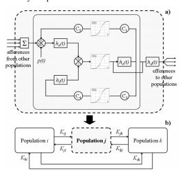
Fig. 1. Structure of the model of multiple coupled neuronal populations. (a) Elementary model for a given population j within (b) the multiple coupled population model. Appropriate setting of parameters  $K_{ij}$  allows for neuronal populations to be unidirectionally and/or bidirectionally coupled. Each population of neurons produces a signal corresponding to local field activity.
