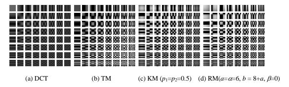
Fig. 16. The basis functions of DCT, TM, KM and RM for block size 8×8.
