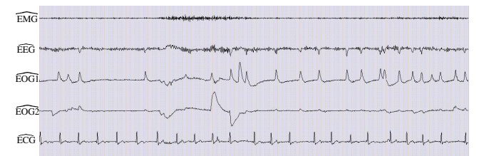
Fig. 6. Separation result of signals depicted in Figure 3(b). \widehat{EMG} is obtained by high-pass filtering. \widehat{EEG} , \widehat{EOG1} , \widehat{EOG2} and \widehat{ECG} are derived using ICA approach and the matching step.
